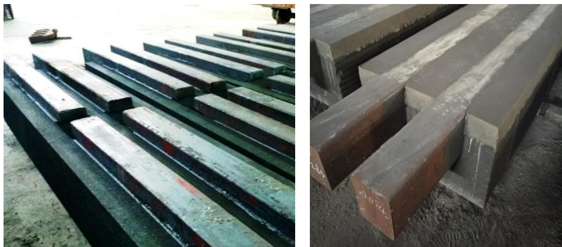
Figure 17. NCCT cathode assembly. Right: after cast iron rodding. Left: ready to be put in a cell.
